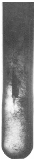
Fig. 2. Pyrolytic char residue within reactor cell following an experiment with Indulin AT Kraft pine lignin polymer.
